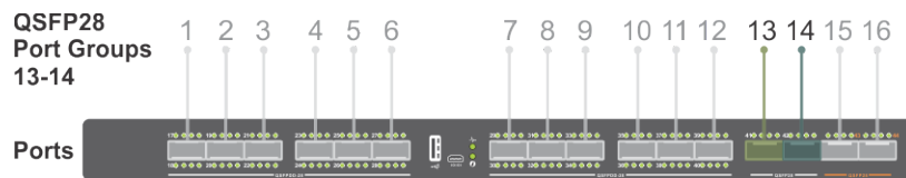
Figure 2. MX9116n Fabric Switching Engine — QSFP28 port groups
