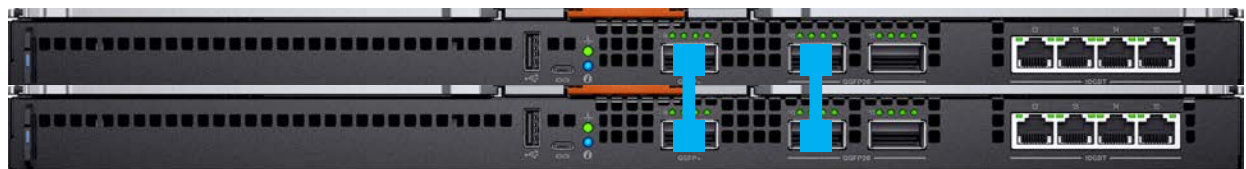
Figure 9 MX5108n SmartFabric VLTi cabling
