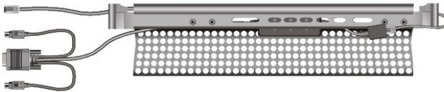
Figure 2-12. 1U or 2U Cable Arm - Top View
