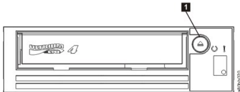
Figure 13. Resetting the Drive
