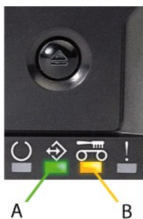
図5: 動作およびClean LED
