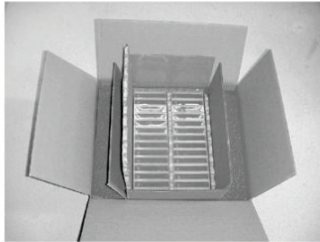
Figure 90. Double-boxing tape cartridges for shipping
