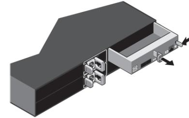
**NOTE:** Before installing the appliance into the rack, it is recommended that you remove the sled(s) for ease of installation.
