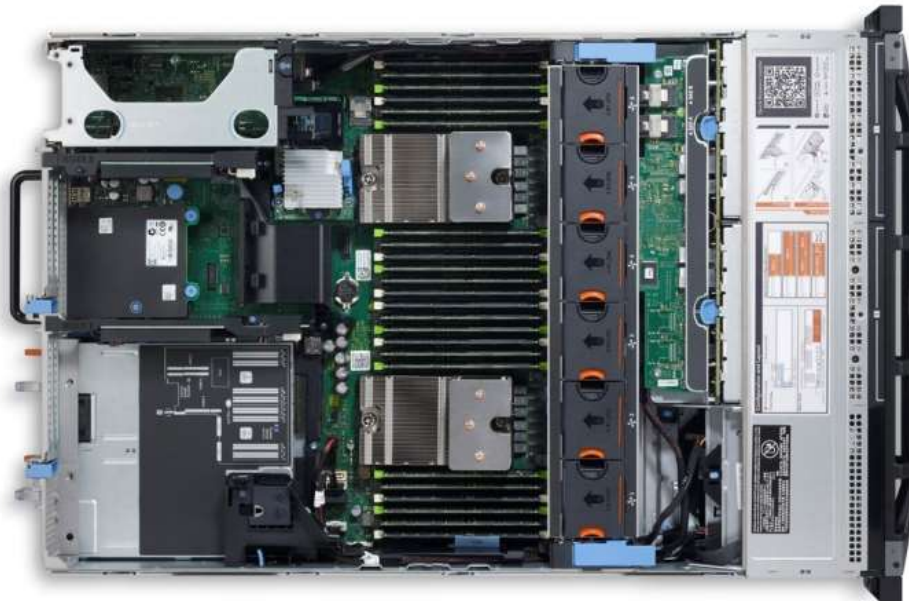
Figure 7. R720 internal chassis view
