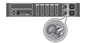
**4** Loop and secure the power cable using the retention strap.
