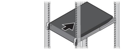
**1** Install the system into a rack.
