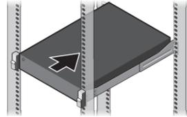
**1** Install the system into a rack.
