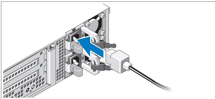
Connect the system's power cable(s) to the system and, if a monitor is used, connect the monitor's power cable to the monitor.
