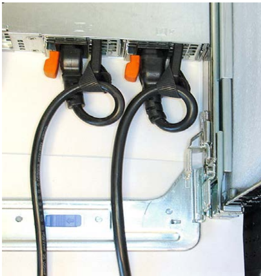
Figure 3: Routing Power Cables Through the Strain Reliefs
