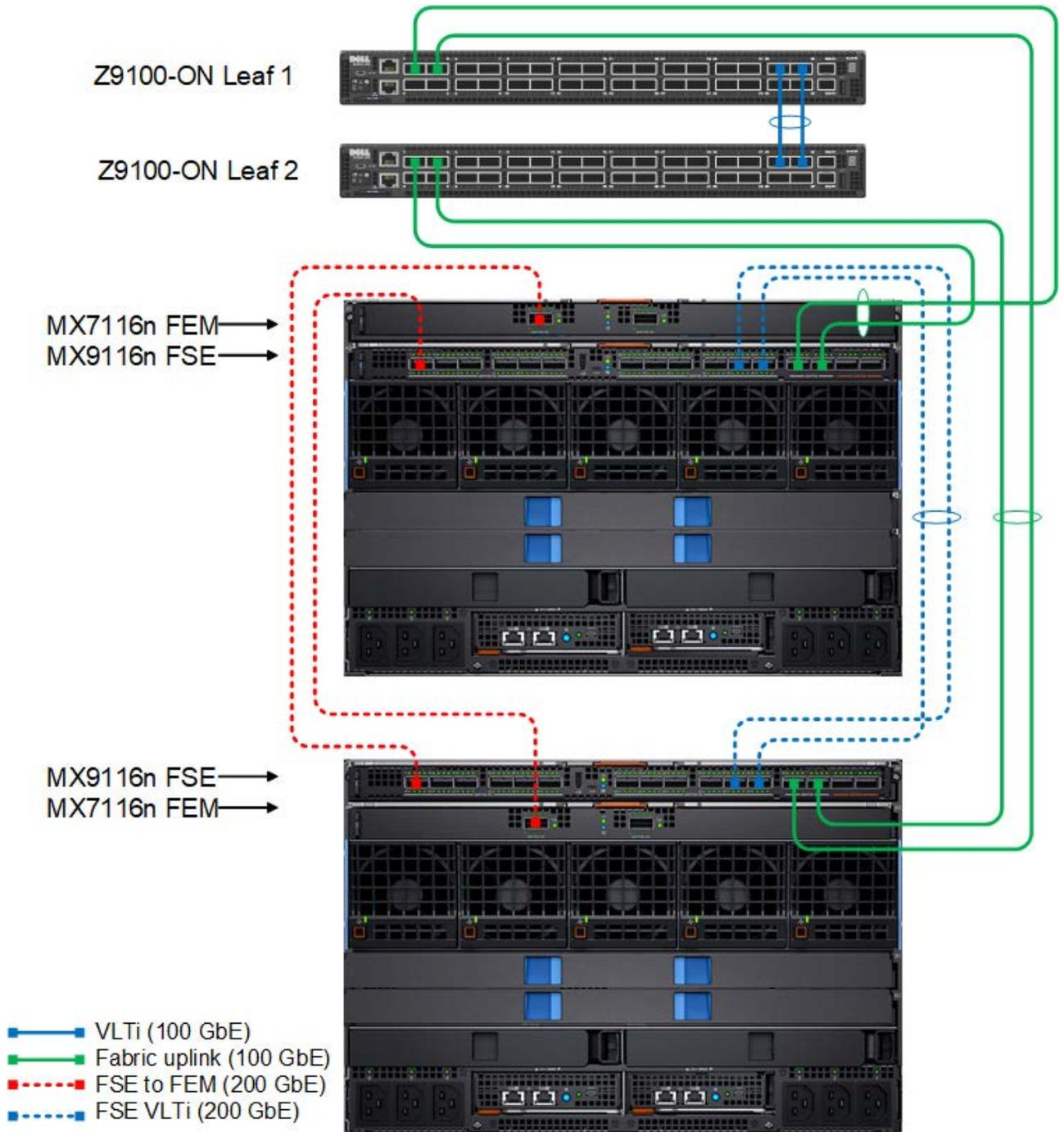
Figure 19 SmartFabric with Z9100-ON leaf switches
