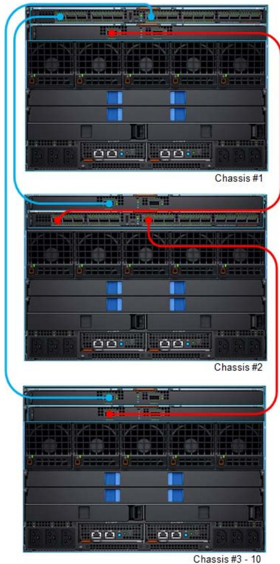
Figure 13 Scalable Fabric example using Fabric A
