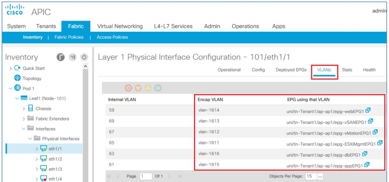
Figure 55 Cisco ACI interface VLANs and EPGs
