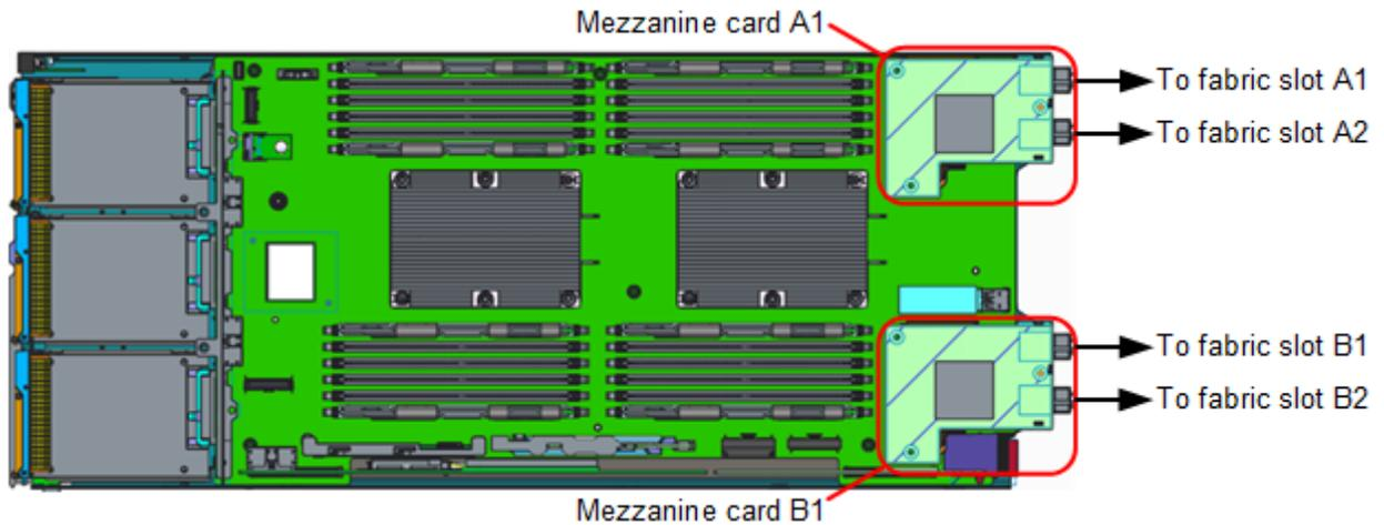
Figure 12 Dell EMC PowerEdge MX740c mezzanine cards
