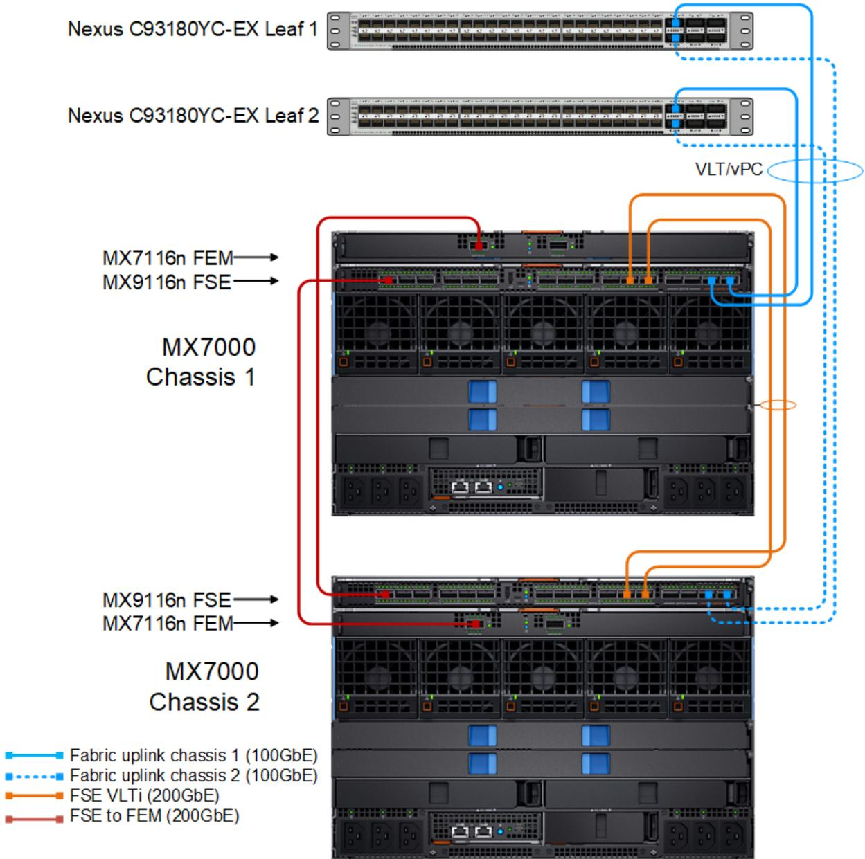
Figure 32 Smart Fabric connected to Cisco ACI leaf switches
