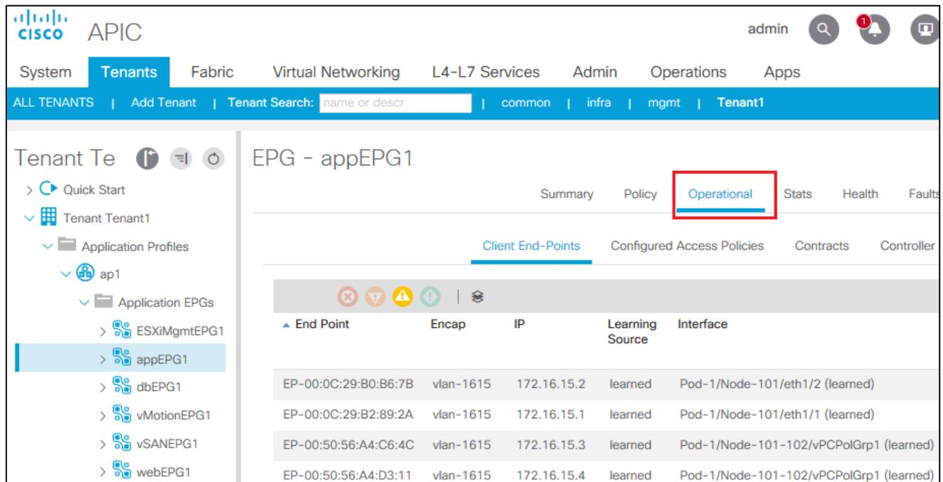
Figure 56 Cisco ACI endpoints in appEPG1
