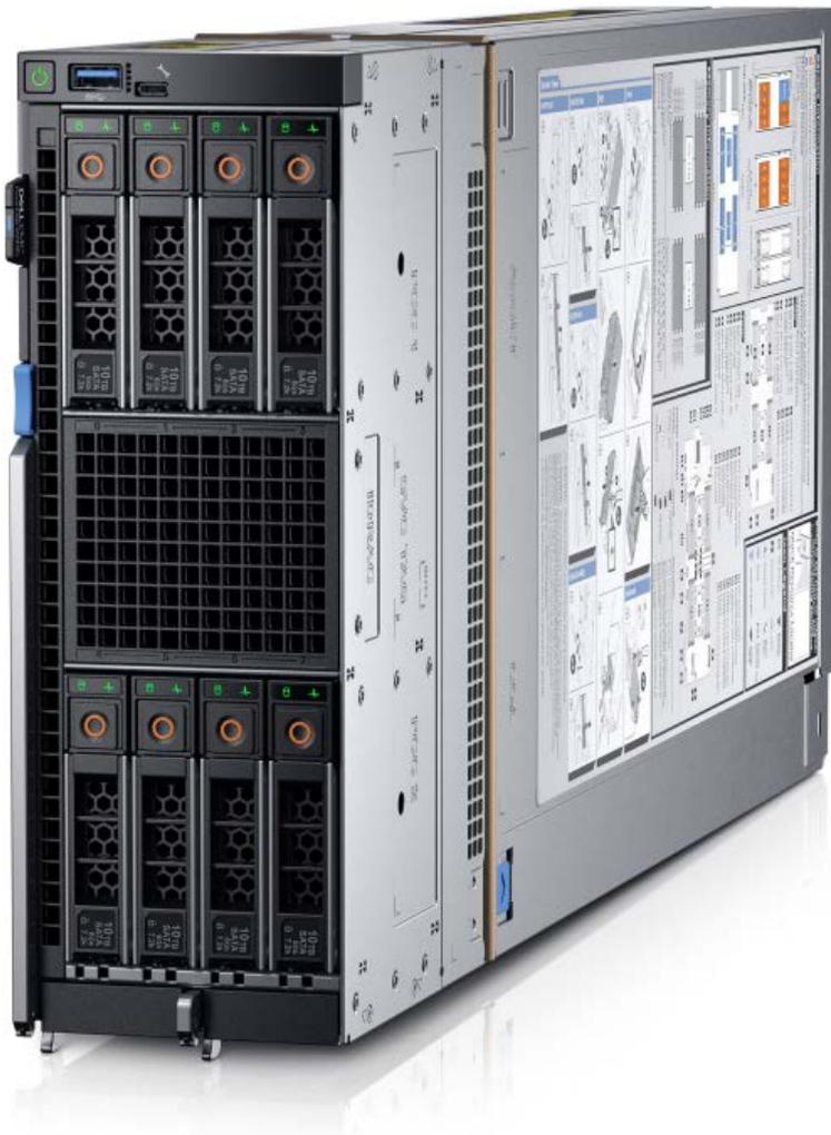
Figure 5 Dell EMC PowerEdge MX840c sled with eight 2.5-inch SAS drives
