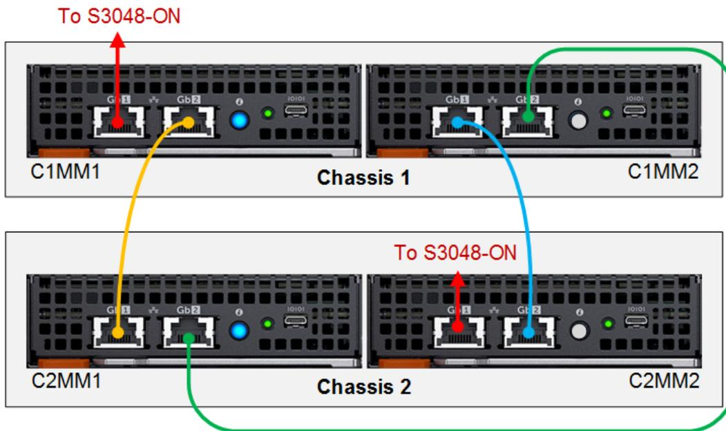
Figure 16 Dell EMC PowerEdge MX9002m module daisy chain cabling
