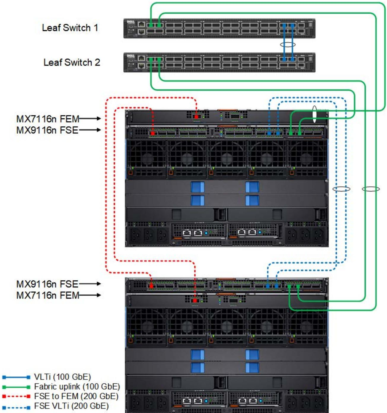
Figure 15 Scalable Fabric Architecture topology
