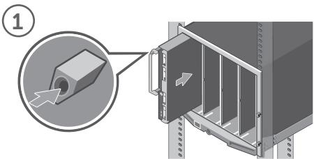
Starting from the left, install the blade(s) into the enclosure.
