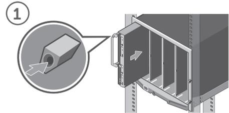
**1** Starting from the left, install the blade(s) into the enclosure.
