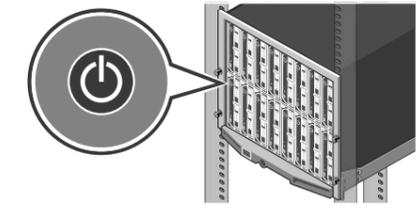
**📄 NOTE:** Ensure that the enclosure is powered on before turning on the blade(s).
