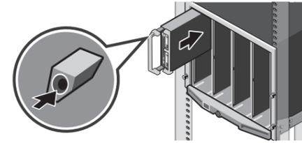
**📄 NOTE:** Beginning from the top, install the blade(s) into the enclosure, from left to right.
