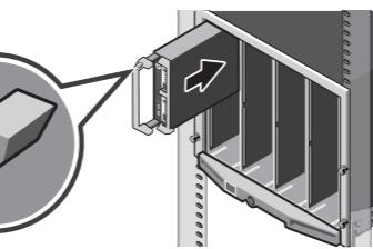
**💡 NOTE:** Beginning from the top, install the blade(s) into the enclosure, from left to right.
