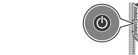
**💡 NOTE:** Ensure that the enclosure is powered on before turning on the blade(s).
