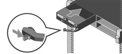
**📌 NOTE:** Beginning from the top, install the sled(s) into the enclosure, from left to right.
