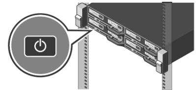
**🔍 NOTE:** Ensure that the enclosure is powered on before turning on the sled(s).
