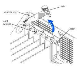
7. To remove the card, grasp the card by the top corners and lift it out.
