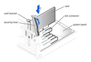
7. Ensure that the card is fully seated in the connector.
