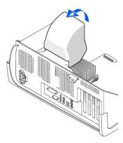
8. For each of the metal securing clips that secure the heat sink to the microprocessor, press down on the clip's latch to release the clip from the retention base. Then lift each clip out of the tabs on the retention base and away from the heat sink.
