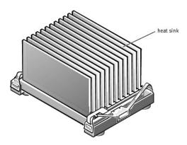
The 478-pin, socketed Intel® Pentium® 4 microprocessor, shown above with the heat sink attached, contains an integrated 8-KB primary (L1) cache with a secondary (L2) 256-KB Advanced Transfer Cache that resides in the processor's core and runs at the processor's internal clock speed.
