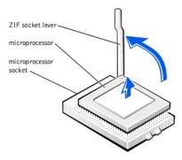
11. Remove the microprocessor from the socket.
