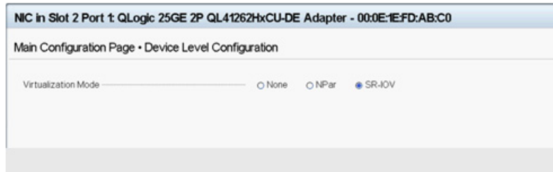
Figure 11-9. System Setup for SR-IOV: Integrated Devices
