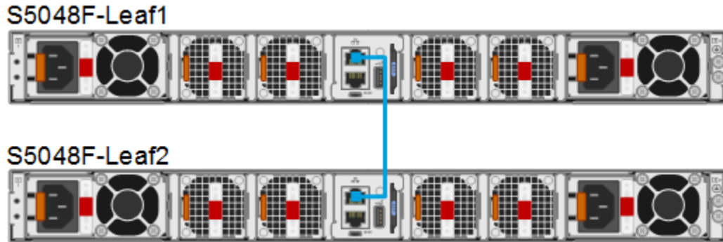
Figure 9 S5048F-ON OOB management interface used for VLT backup destination
