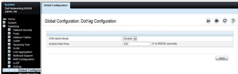
Figure 26-4. Dot1ag Global Configuration
