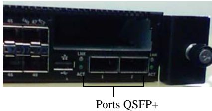
Figure 1. Dell Networking N4000 Panneau avant
