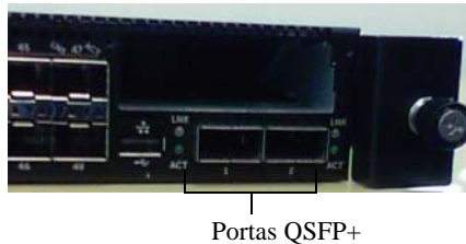
Figura 1. Painel frontal do Dell Networking N4000
