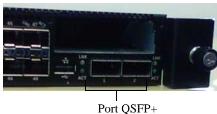
Gambar 1. Dell Networking N4000 Panel Depan
