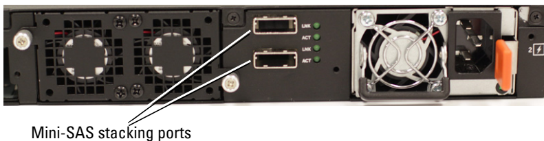
Figure 3-22. Dell EMC Networking N3048ET-ON Mini-SAS Stacking Ports Close-up
