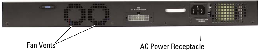
Figure 3-7. Dell EMC Networking N1500 Series Back Panel
