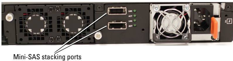
Figure 3-22. Dell EMC Networking N3048/N3048ET-ON Mini-SAS Stacking Ports Close-up
