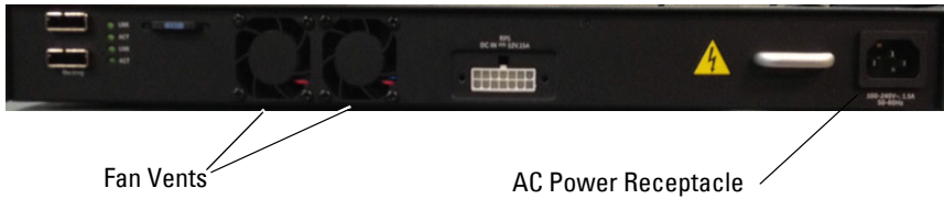
Figure 3-7. Dell Networking N2000 Series Back Panel
