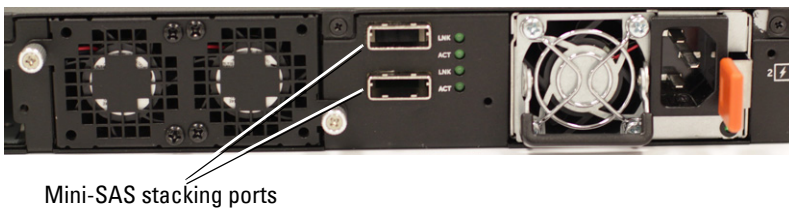
Figure 3-16. Dell Networking N3048 Mini-SAS Stacking Ports Close-up
