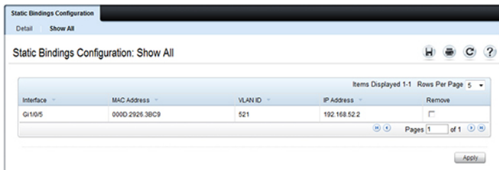
Figure 25-9. DHCP Snooping Static Bindings Summary
