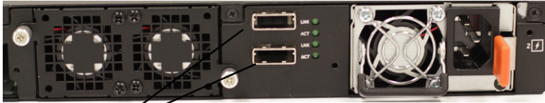
Figure 1-18. N3048 Mini-SAS Stacking Ports Close-up
