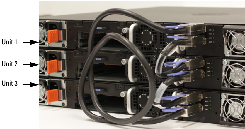
Figure 1-23. Connecting a Stack of Switches
