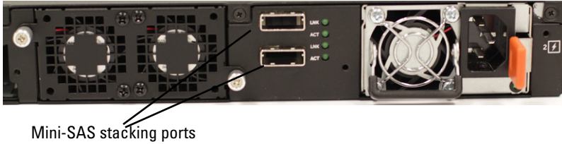
Figure 1-18. N3048 Mini-SAS Stacking Ports Close-up
