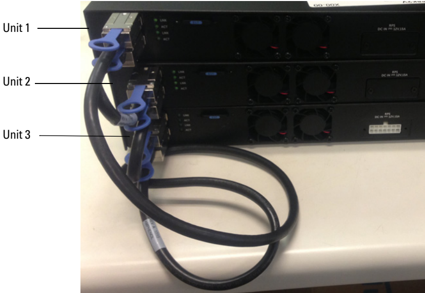
Figure 1-8. Connecting a Stack of Switches
