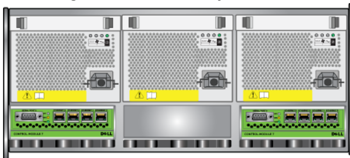
Figure 2-10: PS6500 Array - Rear View
