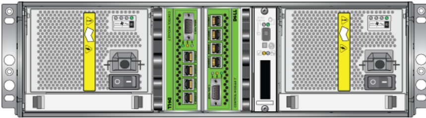
Figure 3-6: Correct Control Module Orientation
