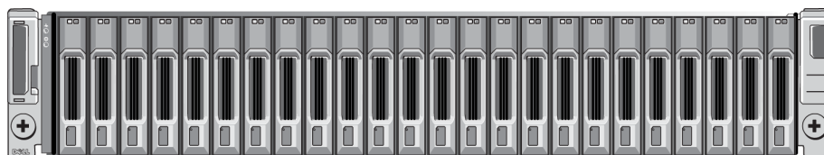
Figure 4: 2.5-Inch Drive Array - Front View (Without Bezel)
