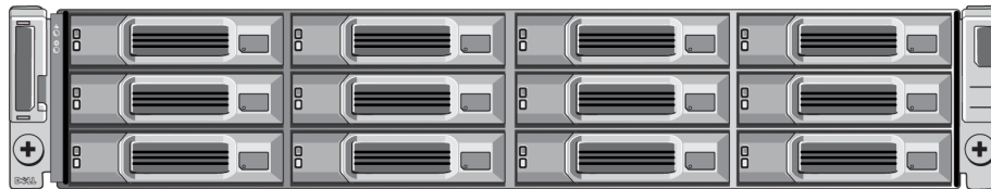
Figure 3: 3.5-Inch Drive Array - Front View (Without Bezel)
