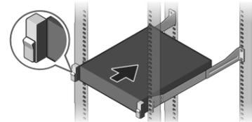
**1** Install the system into a rack.
