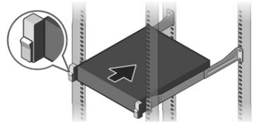
**1** Install the system into a rack.
