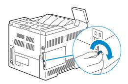
8 Return the cap removed upon installation of the wireless adapter.
