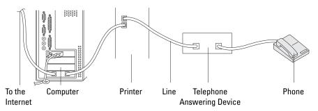
If you want to use your computer modem for faxing or for a dial-up Internet connection, connect the computer modem directly to the back of your printer with the TAD as shown above.
