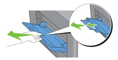
**3** Slide the width guides to the edge of the tray. Th width guides should be fully extended.
