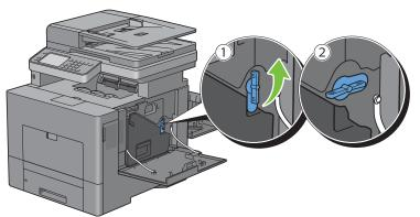
4 Grasp the handle on the waste toner box and pull it out making sure to hold it upright so that the waste toner does not spill out.
