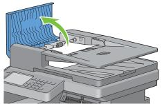
**b** Lift the release lever 90 degrees and remove the jammed document by carefully pulling it to the right.
