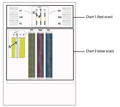
The Chart 1 is used to adjust the color registration for the fast scan direction, which is vertical to paper feed direction. The Chart 2 is used to adjust the color registration for the slow scan direction, which is horizontal to paper feed direction.
