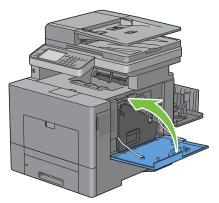
**NOTE:** After replacing the transfer belt unit, be sure to initialize its life counter by following the instructions in the accompanying manual.
