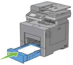
7 Insert the MPF into the printer.
