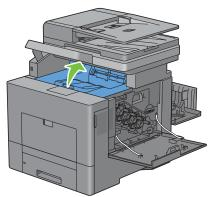
**9** Put your fingers through the loops on both sides of the transfer belt unit, and then pull it out.
