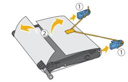
CAUTION: Ensure nothing touches or scratches the surface (black-colored film) of the transfer belt unit. Scratches, dirt, or oil from your hands on the film of the transfer belt unit may reduce print quality.
