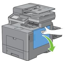
4 Turn the waste toner box lock lever 90-degrees counterclockwise to unlock the waste toner box.
