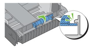
**3** Load paper in trayl, and then insert the tray into the printer and push until it stops.
