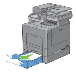
2 Hold the optional 550-sheet feeder with both hands, and remove it from the printer.
