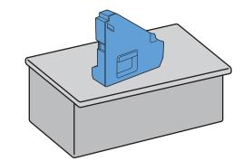
MARNING: Never lay the waste toner box on its side as this may cause its malfunction or toner spills.
