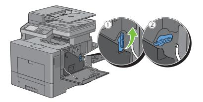
5 Grasp the handle on the waste toner box and pull it out making sure to hold it upright so that the waste toner does not spill out.
