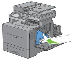
CAUTION: If the waste toner box does not fit into place properly, make sure that the transfer belt unit is fully inserted.
