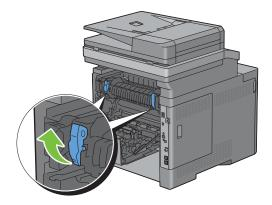
**3** Hold and lower the tab to open the inner part.
