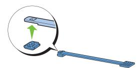
**9** Insert the cleaning rod fully into one of the four holes until it clicks into the interior of the printer as illustrated below, and then pull it out.
