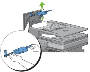
**d** Insert the DADF feed roller assembly and press down the release lever.
