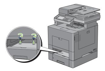
8 Insert trayl into the printer, and push until it stops.
