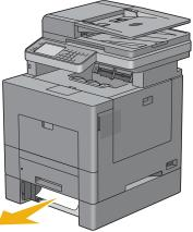
**4** Insert the optional 550-sheet feeder into the printer, and push until it stops.
