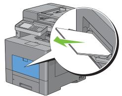
**2** Grasp both sides of the MPF and then pull it out of the printer.
