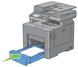
**12** Insert the MPF into the printer.
