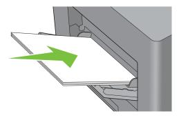
**5** Slide both width guides until they rest lightly against the edge of the print media stack.
