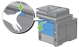
**3** Grasp the grips on both sides of the fusing unit squeezing the lever under the left side grip, and then pull out the unit.
