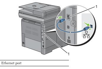
To connect the printer to the network, connect one end of an Ethernet cable into the Ethernet port on the rear of the printer, and the other end to a LAN drop or hub. To setup a wireless connection, insert the wireless adapter into the wireless adapter socket on the back of the printer.
