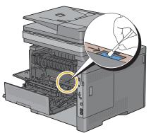
**11** Make sure that the arrow marks on the transfer belt unit and the printer face each other, and then insert the unit into the printer until it clicks.
