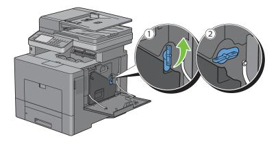
**3** Grasp the handle on the waste toner box and pull it out making sure to hold it upright so that the waste toner does not spill out.
