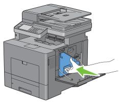
CAUTION: If the waste toner box does not fit into place properly, make sure that the drum cartridge is fully inserted in the previous step.
