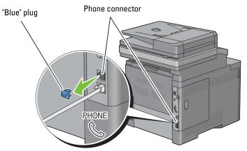
3 To connect a telephone and/or answering machine to your printer, connect the telephone or answering machine line cord into the phone connector (<sup>™</sup>).
