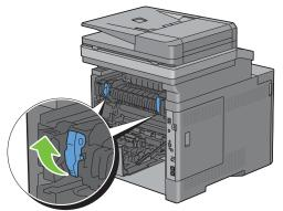
7 Hold and lower the tab to open the inner part.
