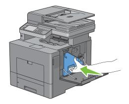
**3** Turn the waste toner box lock lever 90-degrees clockwise to lock the waste toner box.
