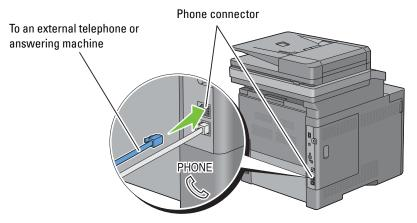
If the phone communication is serial in your country (such as Germany, Sweden, Denmark, Austria, Belgium, Italy, France and Switzerland), and that you are supplied with a "Yellow" terminator, insert the "Yellow" terminator into the phone connector  $\binom{PHONE}{C}$ .
