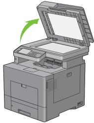
2 Place the document facing down on the document glass and align it with the registration guide on the top left corner of the glass.
