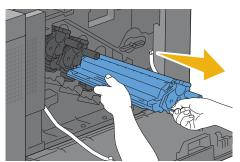
7 Repeat the steps 5 and 6 to remove the other three cartridges.
