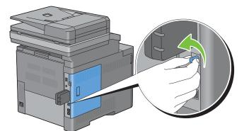
**3** Slide the left side cover towards the back of the printer.
