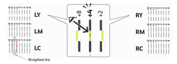
**NOTE:** If it is difficult to choose only one value, as in the case that there seem to be two values closest to a straight line, take the value between the two. For example, in the figure above, -6 and -8 are the values closest to a straight line, so you would enter the value -7.
