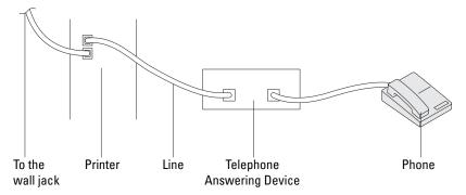
You can connect a telephone answering device (TAD) directly to the back of your printer as shown above.
