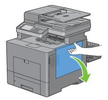
**3** Turn the waste toner box lock lever 90-degrees counterclockwise to unlock the waste toner box.
