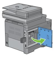
**5** Remove the wireless adapter from the printer by releasing the adapter's hook while pushing the wireless adapter towards the front of the printer.
