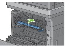
**10** Press down the levers on both sides of the fusing unit, and then close the rear cover.
