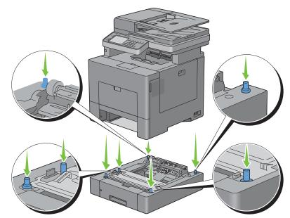
7 Secure the optional 550-sheet feeder to the printer by tightening the two screws provided with the feeder, using a coin or similar object.
