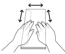
**NOTE:** The maximum height (quantity) of envelopes that can be loaded in the MPF is approximately 15 mm (0.59 inches) (15 envelopes).
