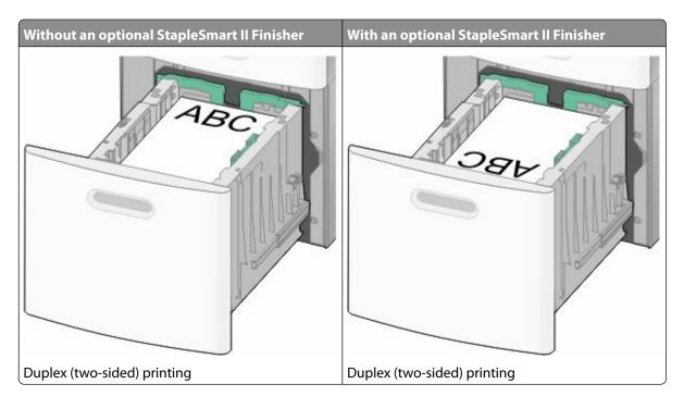
**Note:** Notice the maximum fill line on the side of the tray which indicates the maximum height for loading paper. Do not overload the tray.
