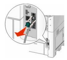
**4** Connect the other telephone cord to a telephone, and then plug it into the EXT port **1** of the printer.
