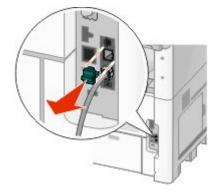
**Note:** Once this plug is removed, any country- or region-specific equipment you connect to the printer by way of the adapter, as shown, will not function properly.
