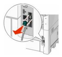
**2** Connect your telecommunications equipment directly to the EXT port **1** on the back of the printer.
