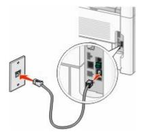
**3** Remove the protective plug from the EXT port **1** of the printer.
