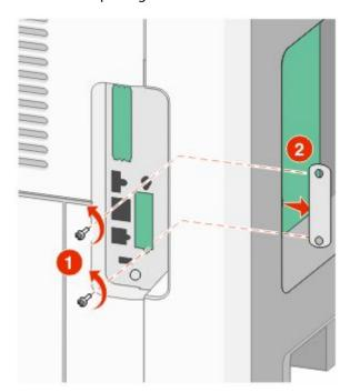
Insert the fax card and attach the two provided screws to secure the fax card mounting bracket.
