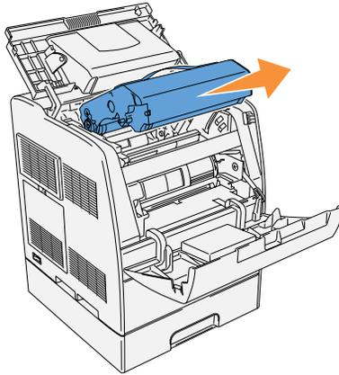
**⚠ CAUTION:** Do not touch inside the printer with your hands. Some parts may be hot. Allow time for the printer to cool before attempting to remove parts in this area.
