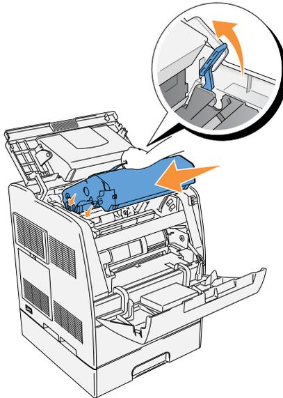
3. Pull down the lever on the right to lock the drum cartridge in place.
