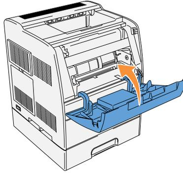
5. Repeat steps 1 through 4 when inserting the remaining cartridges.
