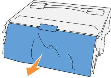
2. Holding the drum cartridge by the handle, align the arrows on the drum cartridge with the corresponding arrows on the printer. Guide the cartridge in until it snaps into place.
