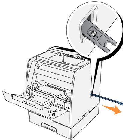
3. Push the two tabs on the cleaning pad inward to remove the pad.
