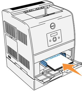
4. Slide the width guides until they rest lightly against the edge of the print media stack.
