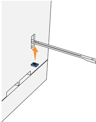
5. Push the cleaning rod back to its original position until it stops.
