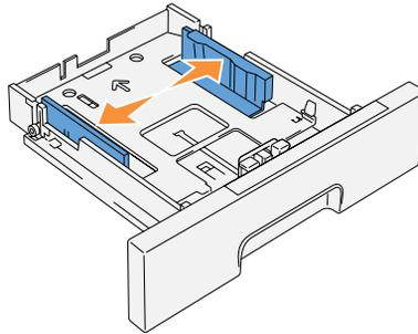
3. Squeeze the length guide and slide it to the edge of the tray.
