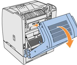
1. To open both covers on the printer, grab the notch in the front door and pull forward. Lift the top cover and push back.
