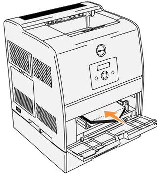
To load envelopes that are under 7.87 inches (220 mm) in width in the multipurpose feeder, insert the envelopes with the flaps open and toward the front of the printer. To load envelopes that are over 7.87 inches (220 mm) in width in the multipurpose feeder, insert the envelopes with the flaps closed and the short-edge of the envelopes facing into the printer. You can load envelopes up to the maximum fill line in the tray at one time.
