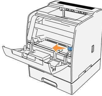
2. Pull the cleaning rod until the cleaning pad comes out of the printer.
