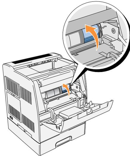
3. Hold the toner cartridge with both hands and pull out the cartridge.
