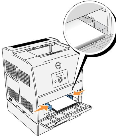
5. Make sure the size and type settings for the multipurpose feeder are set to the correct value for the print media you have loaded.
