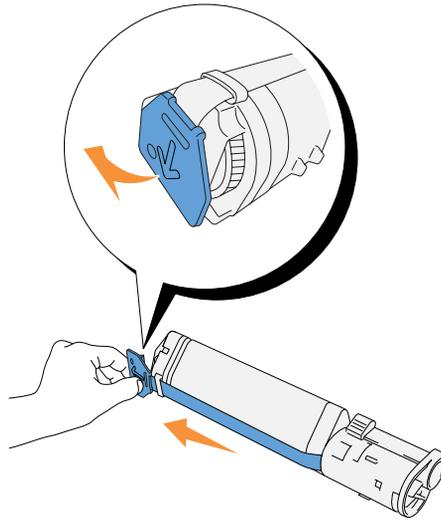
3. To insert the toner cartridge, face the label on the cartridge to the front and align it with the arrows on the printer. Guide the cartridge until it snaps into place and then push down the handhold to lock the cartridge in place.
