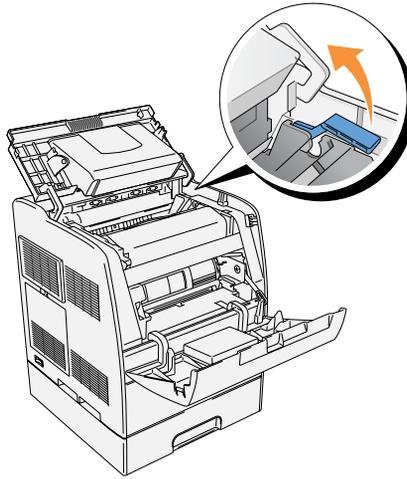
3. Grab the drum cartridge by the handle, and pull it up and out.
