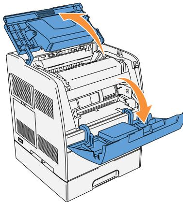
2. To remove the used drum cartridge, push up the lever on the right side of the printer.
