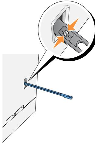
4. Hold the new cleaning pad under the cleaning rod and push it in until it clicks.
