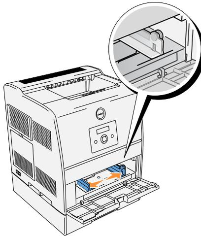
3. Insert the print media into the feeder with the recommended print side face up.
