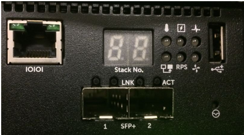
Figure 3-10. Dell EMC Networking N2024/N2048 Close-up
