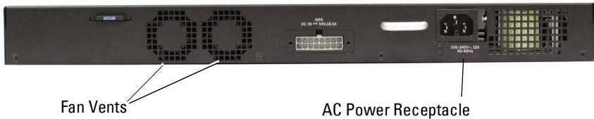
Figure 3-7. Dell EMC Networking N1500 Series Back Panel
