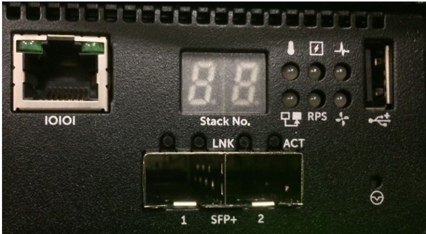
Figure 3-10. Dell EMC Networking N2024/N2048 Close-up
