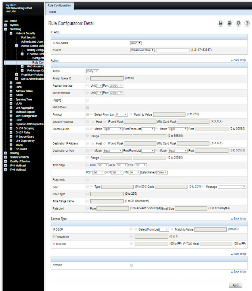
Figure 19-4. IP ACL - Rule Configuration
