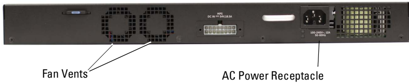
Figure 3-7. Dell EMC Networking N1500 Series Back Panel
