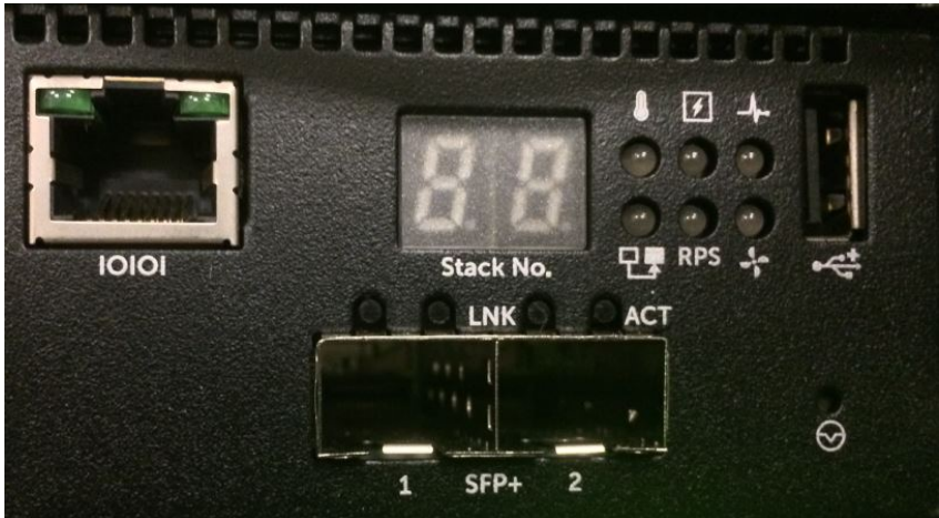
Figure 3-10. Dell EMC Networking N2024/N2048 Close-up
