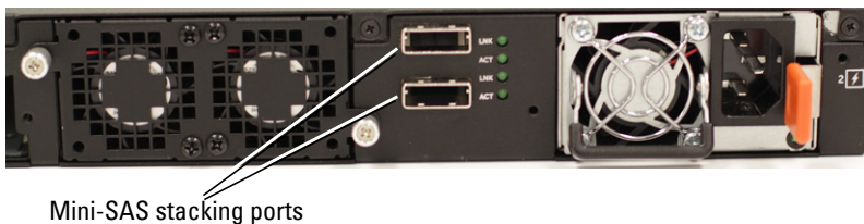
Figure 3-26. Dell EMC Networking N3048ET-ON Mini-SAS Stacking Ports Close-up
