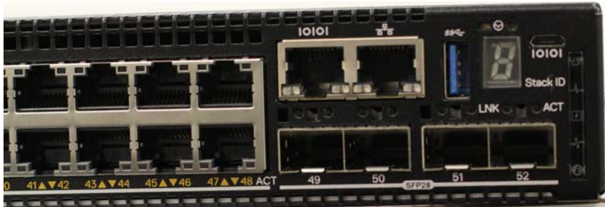
Figure 3-32. Dell EMC Networking N3248 System Panel
