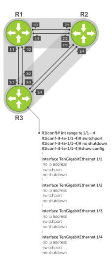
Figure 120. Example of Configuring Interfaces for Layer 2 Mode
