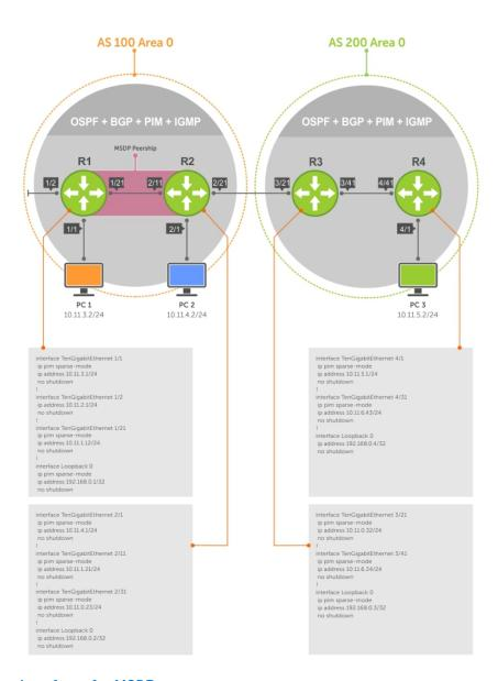
Figure 83. Configuring Interfaces for MSDP
