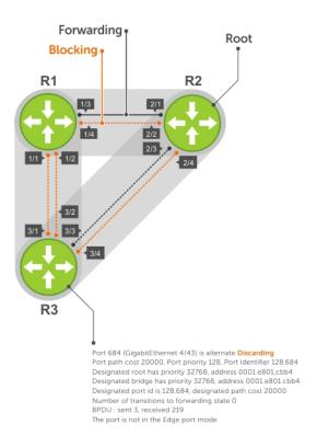
Figure 112. Rapid Spanning Tree Enabled Globally
