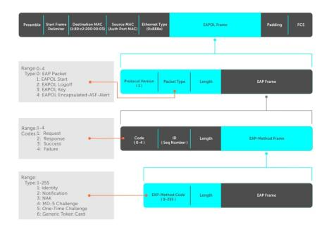
Figure 4. EAP Frames Encapsulated in Ethernet and RADUIS
