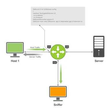
Figure 100. Port Monitoring Example
