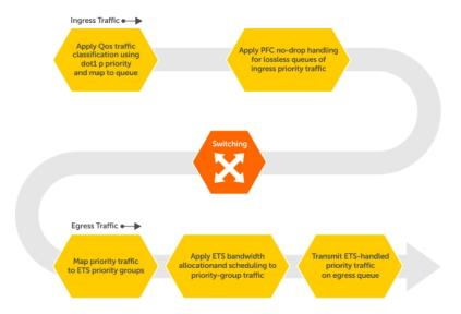
Figure 31. DCB PFC and ETS Traffic Handling
