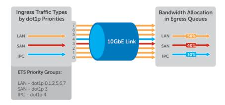
Figure 30. Enhanced Transmission Selection
