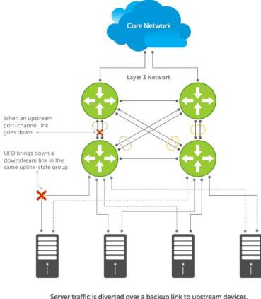
Server traffic is diverted over a backup link to upstream devices.
