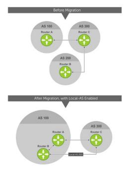
Figure 22. Before and After AS Number Migration with Local-AS Enabled
