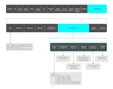
Figure 45. IGMP Version 3-Capable Multicast Routers Address Structure
