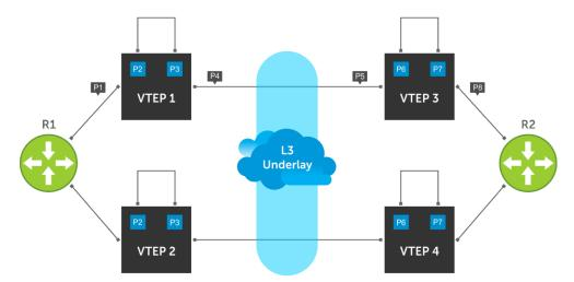
In this topology, P2 and P3 in VTEP 1 are VLT port-channels with corresponding VLT peer LAGs being P2 and P3 in VTEP 2. Similarly, P6 and P7 in VTEP 3 are VLT port-channels with corresponding VLT peer LAGs being P6 and P7 in VTEP 4.
