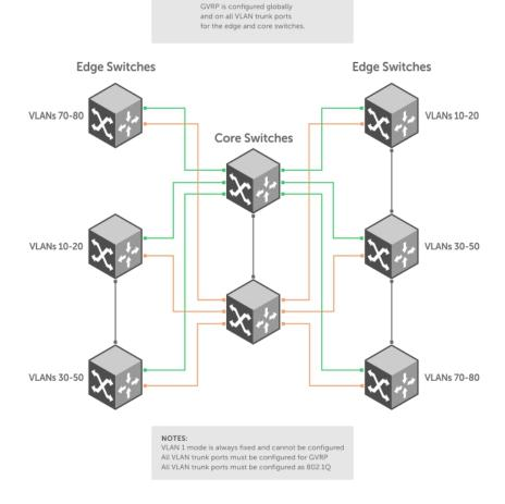
Figure 42. Global GVRP Configuration Example
