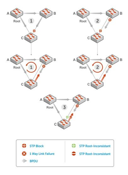
Figure 124. STP Loop Guard Prevents Forwarding Loops
