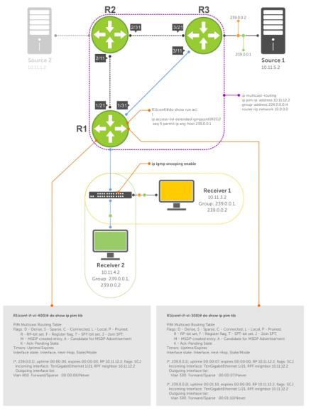
Figure 93. Preventing a Host from Joining a Group
