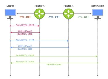
Figure 56. Path MTU discovery process
