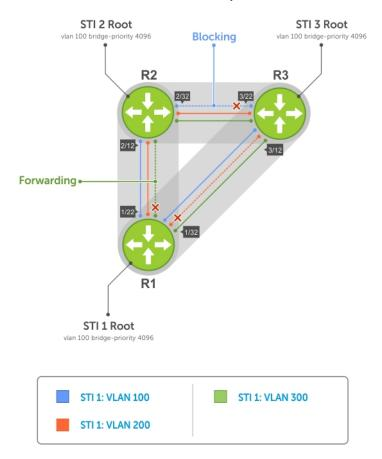
Figure 106. Load Balancing with PVST+
