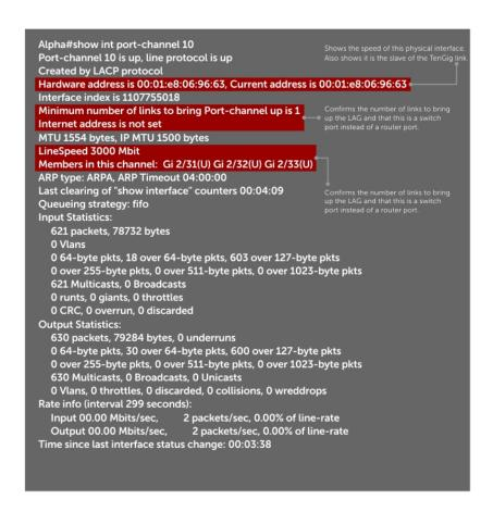
Figure 65. Inspecting Configuration of LAG 10 on ALPHA
