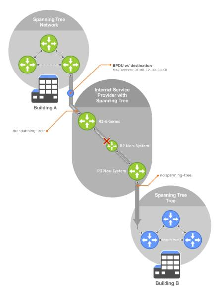
Figure 118. VLAN Stacking without L2PT
