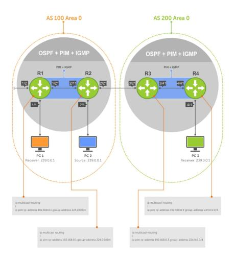
Figure 85. Configuring PIM in Multiple Routing Domains
