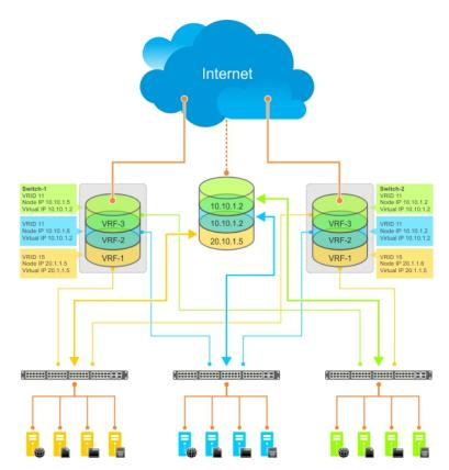
Figure 173. VRRP in a VRF: Non-VLAN Example
