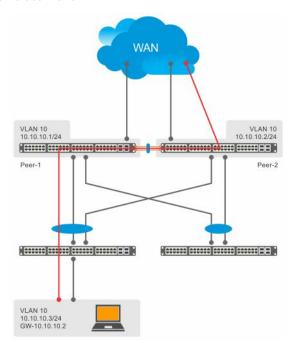
Figure 137. Packets without peer routing enabled
