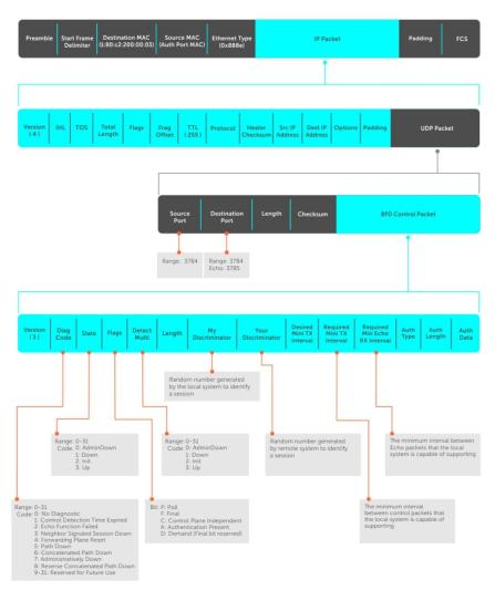
Figure 9. BFD in IPv4 Packet Format
