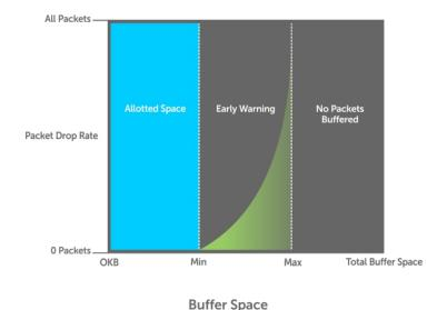
Figure 110. Packet Drop Rate for WRED
