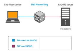
Figure 3. EAP Frames Encapsulated in Ethernet and RADUIS
