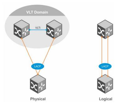
Figure 131. VLT providing multipath
