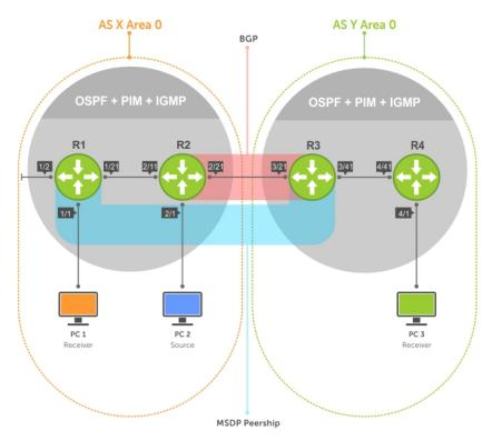
Figure 81. Multicast Source Discovery Protocol (MSDP)
