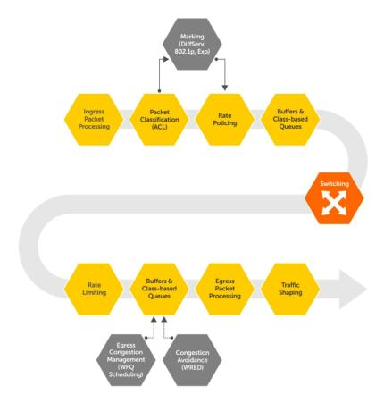
Figure 108. Dell EMC Networking QoS Architecture
