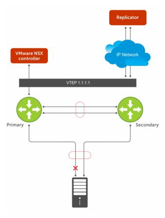
Figure 159. Controller-based VXLAN for VLT Providing Redundancy
