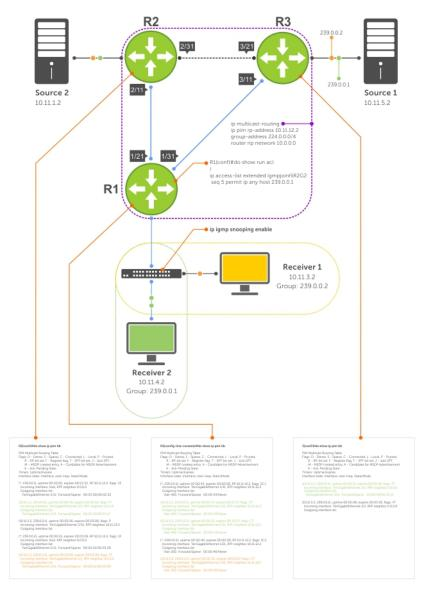
Figure 94. Preventing a Source from Transmitting to a Group
