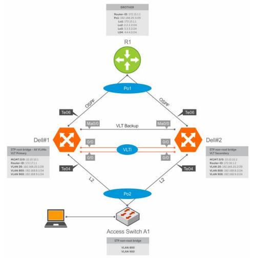
Figure 139. Peer Routing Configuration Example
