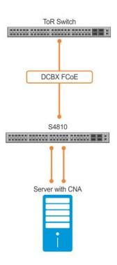
Figure 38. Configuration Example: FIP Snooping on a Switch
