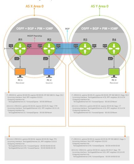
Figure 90. MSDP with Anycast RP
