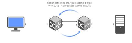
Use backup interfaces to create redundant links in networks without STP
