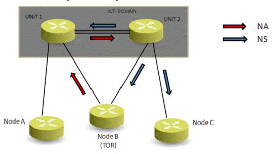
Figure 141. Sample Configuration of IPv6 Peer Routing in a VLT Domain
