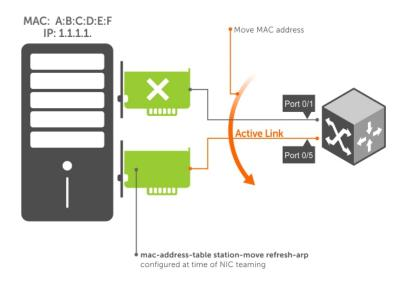
Figure 71. Configuring the mac-address-table station-move refresh-arp Command
