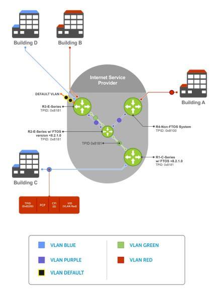
Figure 115. Single and Double-Tag First-byte TPID Match
