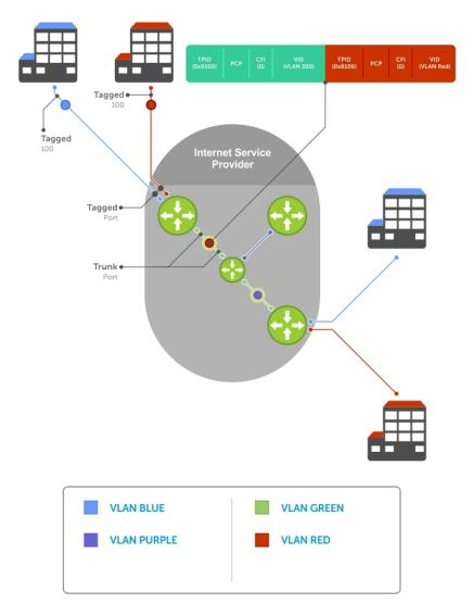
Figure 113. VLAN Stacking in a Service Provider Network
