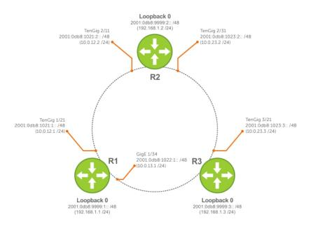
Figure 60. IPv6 IS-IS Sample Topography
