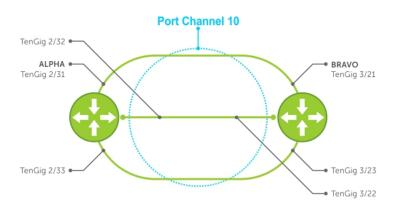
Figure 63. LACP Basic Configuration Example
