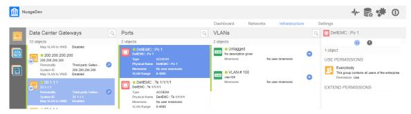
Figure 156. Port-to-VLAN mappings
