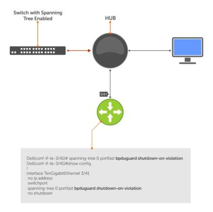
Figure 122. Enabling BPDU Guard
