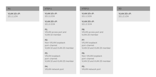
In this RIOT scheme, whenever R1 tries to reach R2, the packet gets to P1 on VTEP 1 with VLAN 10 and gets routed out of P2 on VLAN 20. VTEP 1 sends an ARP request for R2 (10.1.2.1) through P2. This request gets VXLAN encapsulated at P3 and is sent out of P4. Eventually, the native ARP request reaches R2.
