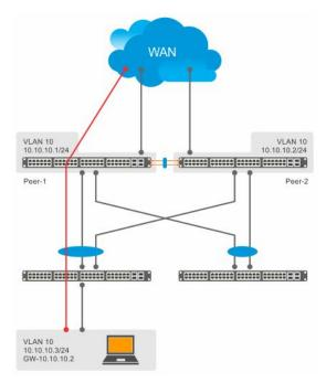
Figure 138. Packets with peer routing enabled
