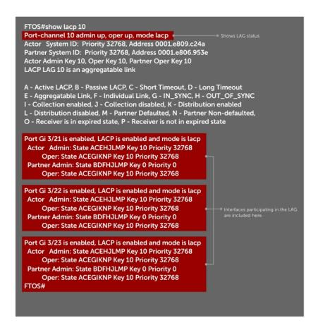
Figure 69. Inspecting the LAG Status Using the show lacp command
