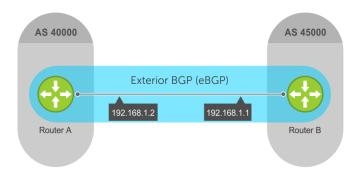
Figure 23. BGP topology with two AS
