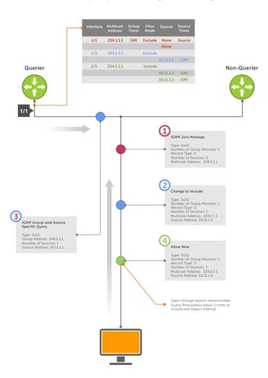
Figure 46. Membership Reports: Joining and Filtering
