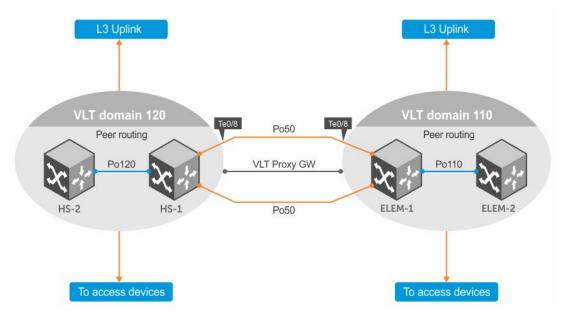
Figure 145. VLT Proxy Gateway Sample Topology
