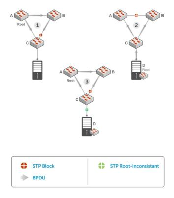
Figure 123. STP Root Guard Prevents Bridging Loops
