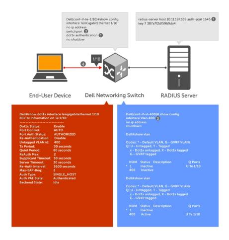
Figure 8. Dynamic VLAN Assignment
