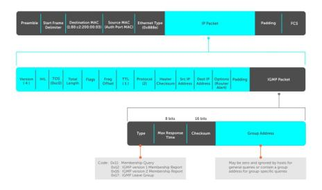
Figure 43. IGMP Messages in IP Packets
