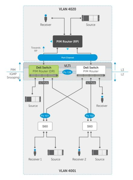
Figure 136. PIM-Sparse Mode Support on VLT
