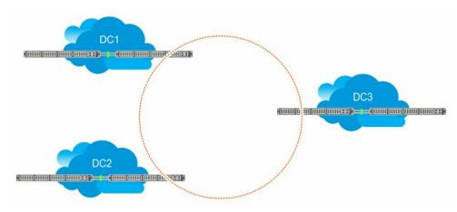
Figure 40. FRRP Ring Connecting VLT Devices
