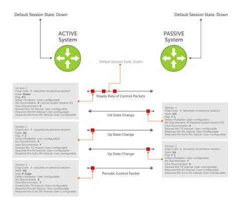
Figure 10. BFD Three-Way Handshake State Changes
