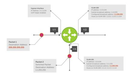
Figure 54. UDP Helper with Configured Broadcast Addresses
