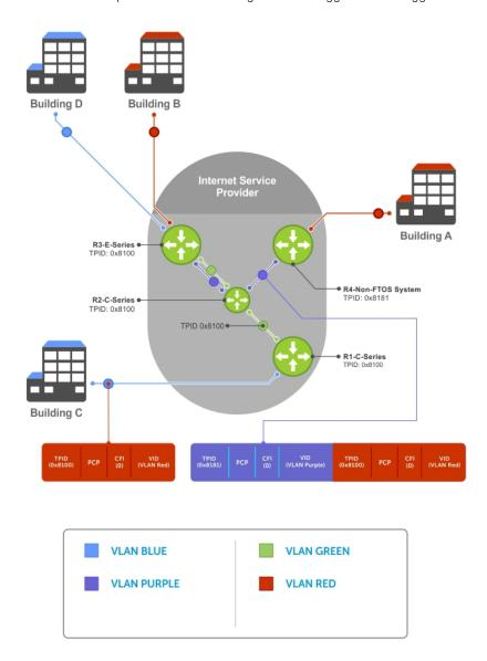
Figure 114. Single and Double-Tag TPID Match
