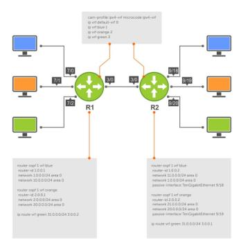
Figure 168. Setup OSPF and Static Routes
