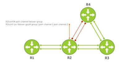
Figure 62. Configuring Shared LAG State Tracking
