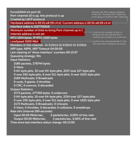
Figure 68. Inspecting LAG 10 Using the show interfaces port-channel Command
