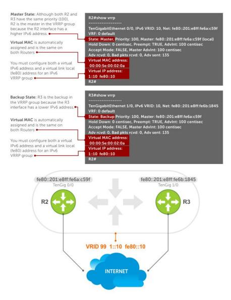
Figure 172. VRRP for an IPv6 Configuration
