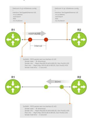
Figure 73. Configuring Far-End Failure Detection
