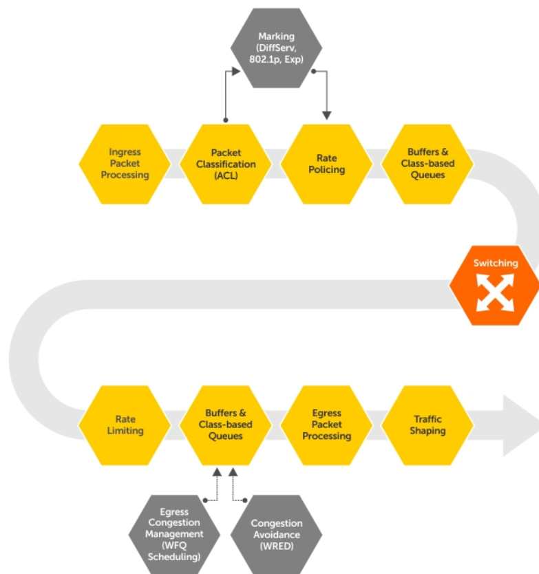
Figure 111. Dell EMC Networking QoS Architecture
