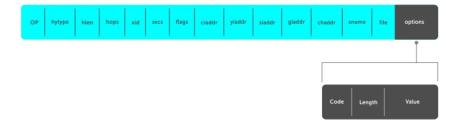
Figure 34. DHCP packet Format
