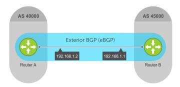
Figure 23. BGP topology with two AS
