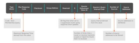
Figure 47. IGMP Version 3 Packet Structure
