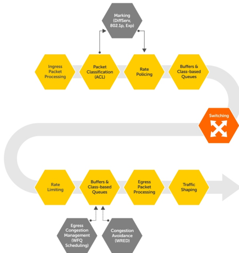
Figure 108. Dell EMC Networking QoS Architecture
